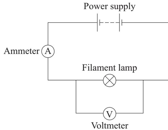
Name a component connected in parallel with the filament lamp.
